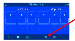
Press the "X" button to delete the switching time.
