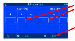
By pressing the corresponding buttons, the day of the week, hour and minute are entered for the switch-on time and the switch-off time.
